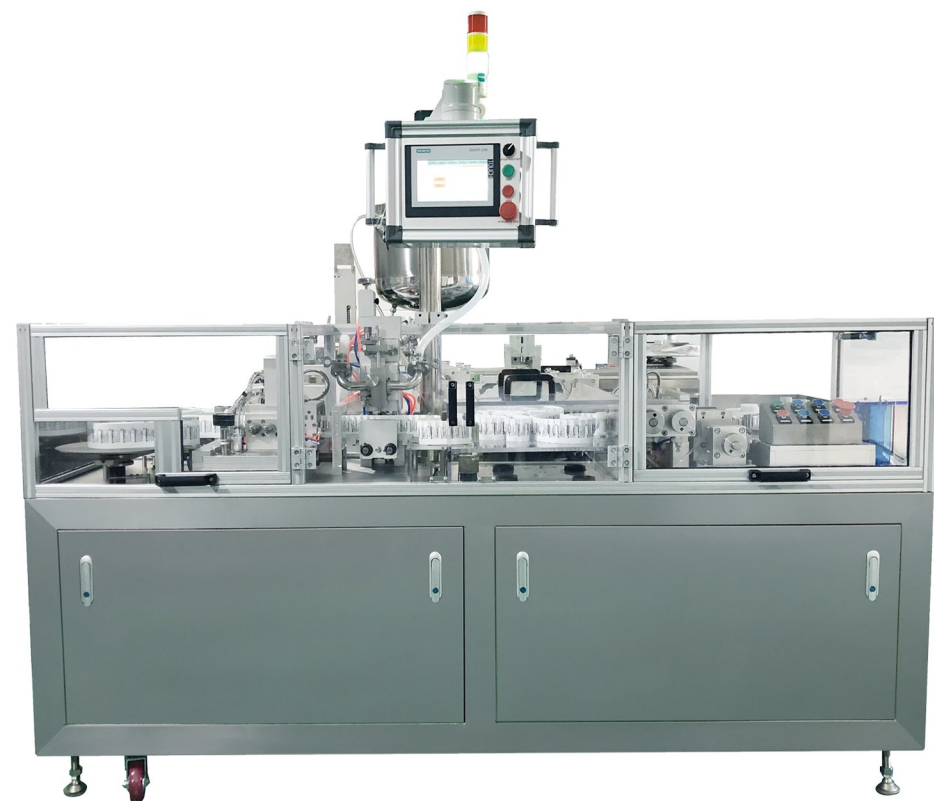
SupLab-I Automatic suppository Pproduction line
